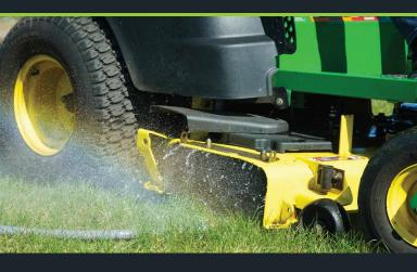
Keeping your lawn mower deck free of debris is an important part of proper equipment maintenance.
